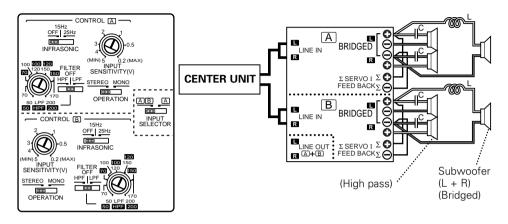
• Principle of Tri-mode Method of frequency band division using a coil and capacitor…in case of 6dB/oct. slope
